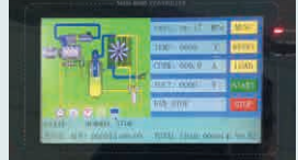
REAL-TIME DIAGNOSTIC COLOUR DISPLAY INDICATES COMPRESSOR STATUS
