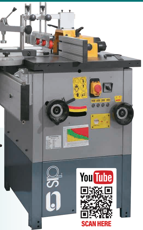
Spindle Moulder shown with optional sliding carriage (01457)
