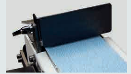
ADJUSTABLE TOOL SUPPORT; FOR ACCURATE POSITIONING OF THE WORKPIECE WITH ANGLE ADJUSTMENT
