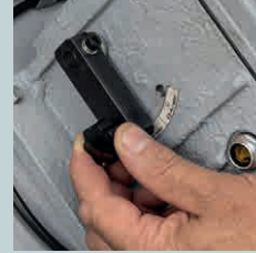
DIRECT DRIVE MOTOR GEARBOX WITH 3 SPEED QUICK-CHANGE SWITCH FOR EASY BLADE CUTTING SPEED SELECTION
