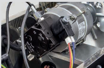
DANFOSS FUEL PUMP INSTALLED
