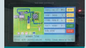
REAL-TIME DIAGNOSTIC COLOUR DISPLAY INDICATES COMPRESSOR STATUS
