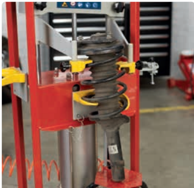
Fast and safe compression of road springs.
