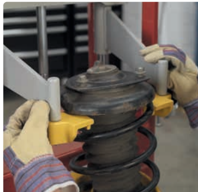
Air operated unit with safety locking guard.
