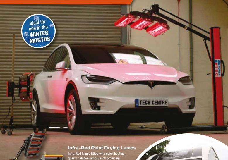
quartz halogen lamps, each providing 1000w of power. Ideal for spot repairs, engine drying, adhesive strip removal, drying filler or primer, or pre-heating prior to spraying. Their low chassis & tall frames allow for work to be undertaken on all parts of the vehicle.
