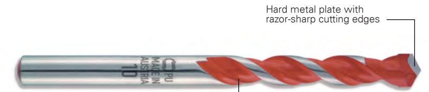
4-fold volume drill spiral for quick drill dust removal
